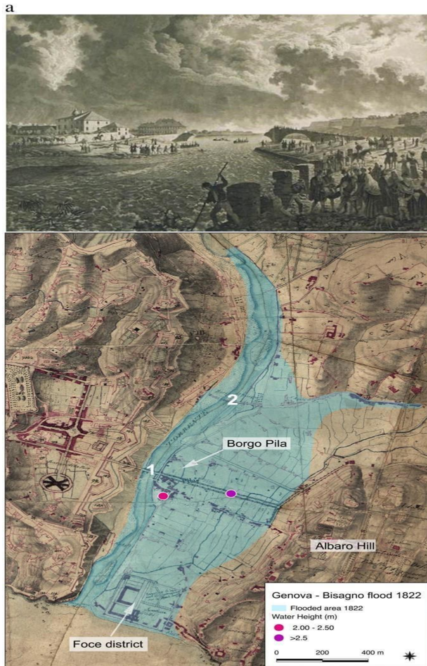
Fig. 12, The Genoa flood of 1822 the Bisagno stream flooded the natural alluvial plain designated to it which had not yet been urbanized and is now unrecognizable. On that day, 812 millimetres of rain fell in 24 hours. 199
